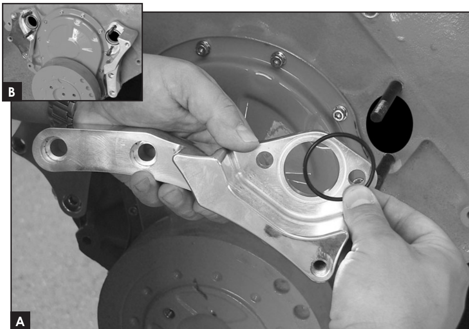
Figure 3: Install Alternator Bracket
