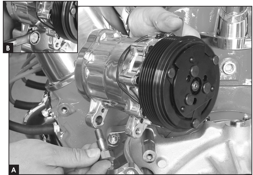
Figure 8: Install SD-7 Compressor
