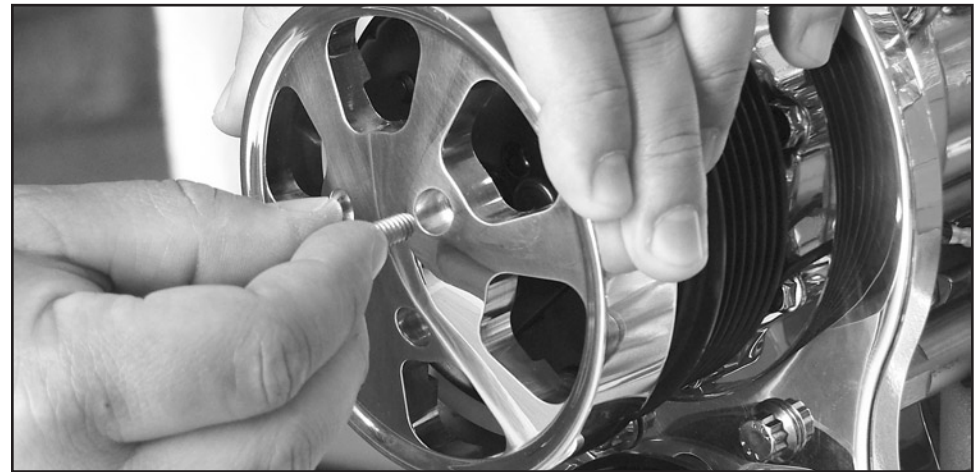
Figure 13: Install SD-7 Compressor Clutch Cover
