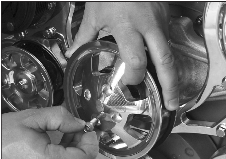
Figure 11: Install Water Pump Pulley onto Pump
