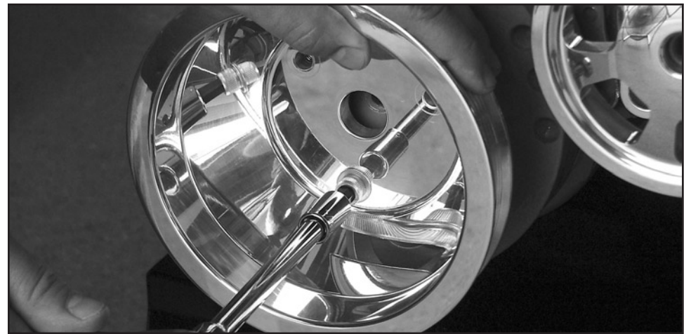
Figure 12: Install Crankshaft Pulley
