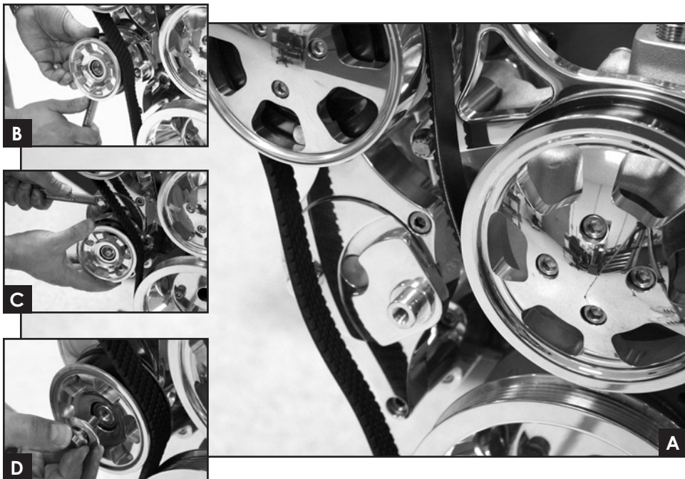
Figure 14: Install Serpentine Belt & Tensioner Pulley
