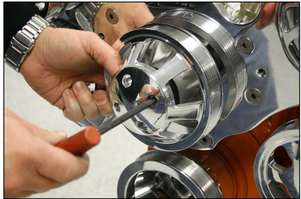
Figure 12: Install Water Pump Pulley
