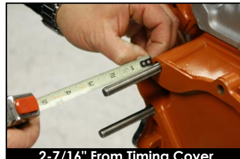
Figure 2: Install Block Mounting Studs
