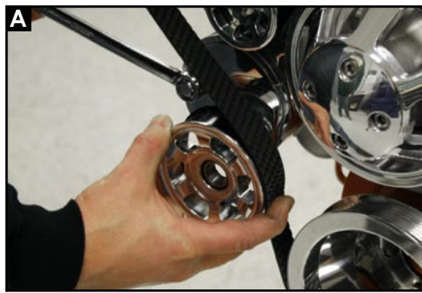
Figure 15: Install Belt & Tensioner Pulley
