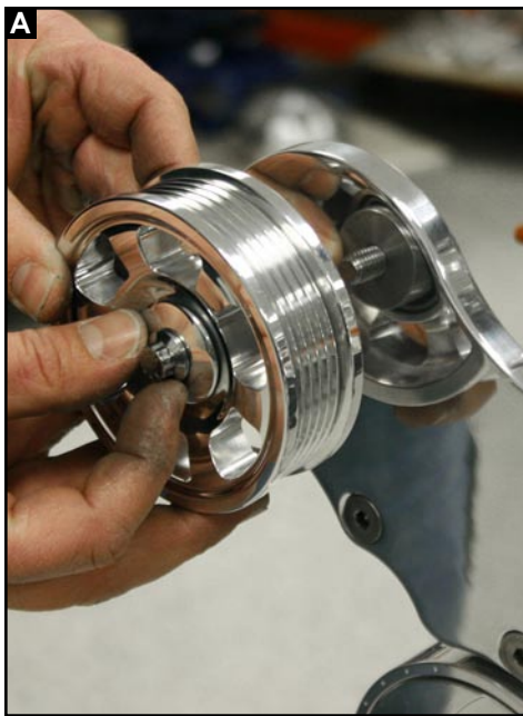
Figure 13: Install Idler Pulleys
