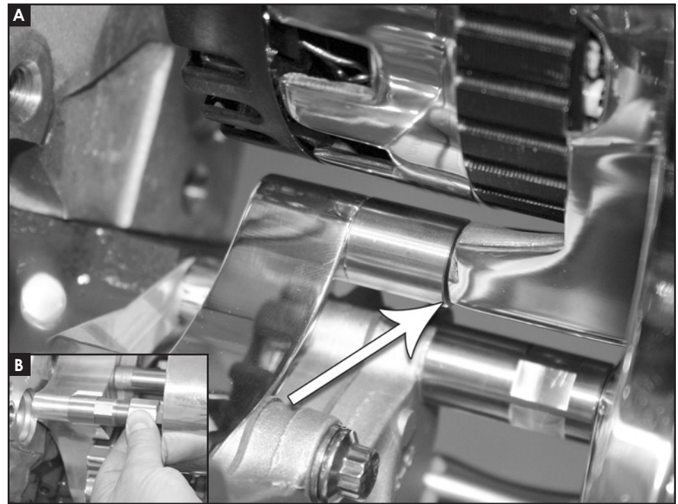
Figure 17: Complete Bridge Bracket Installation
