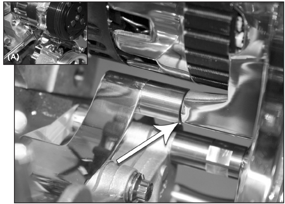
Figure 18: Complete Bridge Bracket Installation
