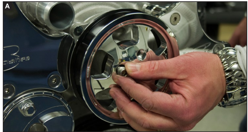
Figure 7: Install Water Pump Pulley
