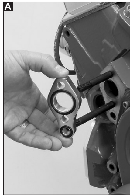
Figure 2: Install Water Pump Spacer & Alternator Bracket
