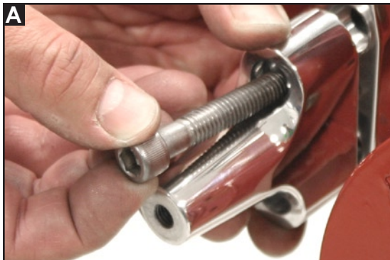
Figure 4: Install Lower Tensioner Bracket
