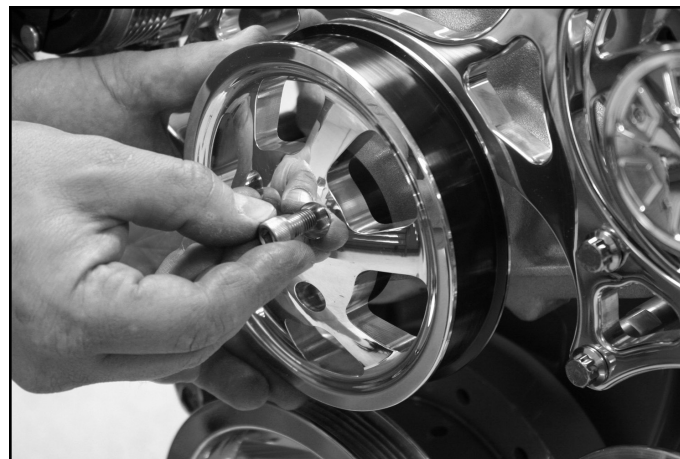
Figure 12: Install Water Pump Pulley
