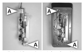
**65. Verify the shifter mechanism is free of any debris** and loose hardware. Remove the shift knob, and place the tower over the shifter. Align the tower's through-holes with the outboard screw holes on the shifter's front and rear brackets (at locations "A").
