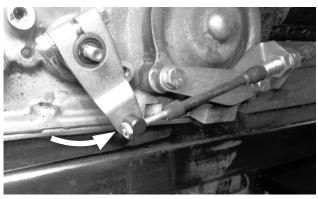
**37.** With the swivel still in the selector lever, operate the shifter through each position, verifying that the swivel slips freely in and out of the lever in each position.
