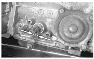
**29.** If the stock selector lever points generally downward, cut it off at the inboard bend, in order to allow the B&M lever to be positioned correctly.
