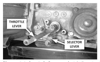
**27. Disconnect stock controls:** Remove and retain the nut and lock washer holding the throttle lever on its shaft. Carefully remove the throttle lever, and move it and its linkage aside, allowing them to hang free. Remove and discard the stock shift linkage.
