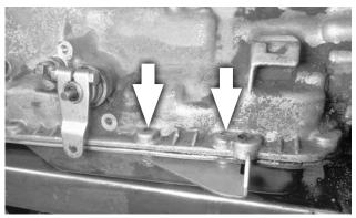
B. <u>C6 transmissions</u>: Install the cable bracket at the two left rear oil pan bolt holes, using the two 5/16-18 × 1" bolts and flat washers. For stamped sheet-metal (stock) pans, use the two spacers between the pan and bracket. (Spacers are not used with cast aluminum pans.) Tighten the bolts to 12-13 ft-lbs torque.
