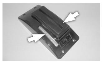
**64. Install** the **shifter boot** and the appropriate **indicator window** in the **tower cover**. (Use the 4-speed window for GM 4-speed transmissions only; use the 3-speed window for all others, including 4-speed Chryslers and Fords.)
