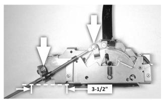
7. Assemble the cable and shifter. Secure the cable eye to the shifter pin with a 1/4" I.D. e-clip. Then secure the cable's mount tab to the outside surface of the shifter base with the 1/4-20 × 1/2" bolt and a 1/4" nut (apply medium strength thread-locking fluid to the bolt).
