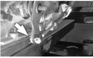
**38.** Secure the swivel to the selector lever with the cotter pin. Operate the shifter through all the gear positions, verifying that it operates correctly.
