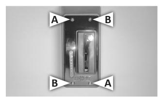
66. Place the assembled cover over the shift lever and tower.
