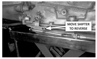
53. With the swivel still in the selector lever, lift the shifter lever and push it forward 2 clicks to REVERSE. Verify that the swivel still slips freely in and out of the selector lever. If not, adjust the large cable nuts (and the swivel, if necessary) until it does.
