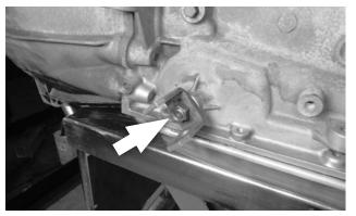
**44. Disconnect stock controls:** Remove and retain the selector lever nut. Remove and discard the selector lever and shift linkage.
