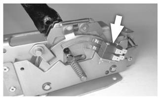
8. Install the two micro-switches on the shifter mechanism as shown, using the two #4-40 × 1-1/4" screws, lock washers and nuts.
