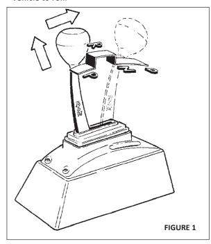
**To get to REVERSE** (whether from PARK, NEUTRAL or DRIVE), lift the lever to clear the Reverse Lockout and move the stick to the REVERSE position.
