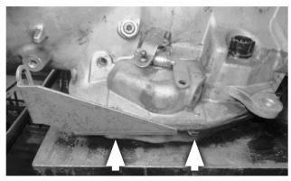
14. Install the cable bracket at the two pan bolt holes directly below the selector lever, using the two 5/16-18 × 1" bolts and flat washers. For stamped sheet-metal (stock) pans, use the two spacers between the pan and bracket. (Spacers are not used with cast aluminum pans.) Tighten the bolts to 12-13 ft-lbs torque.
