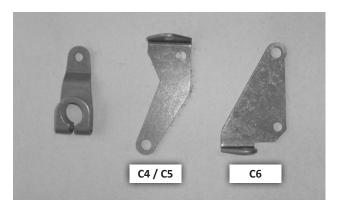
**26. Get the Ford selector lever and appropriate cable bracket** from the parts kit.
