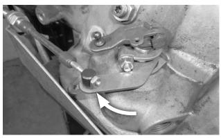
**20.** With the swivel still in the selector lever, operate the shifter through each position, verifying that the swivel slips freely in and out of the lever in each position.
