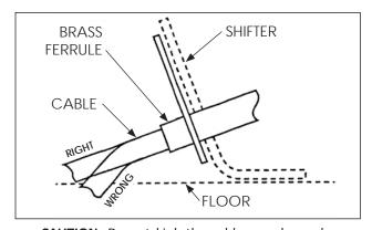
**CAUTION:** Do not kink the cable anywhere along its length, or it will lock up. The cable should be kept straight for at least 2" after it leaves the brass ferrule at each end.
