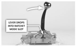
50. On the transmission, manually move the selector lever to the DRIVE detent (that is, 3 clicks back from full-forward / PARK). Then in the vehicle, move the shifter to the DRIVE position (4 clicks back from full-forward; the shift lever will drop into the ratchet mode slot).
