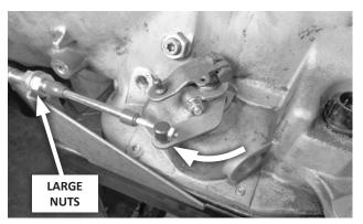
17. Manually move the selector lever to the LOW (full-forward) detent. Move the shifter handle to the LOW position (ratcheted all the way back). Adjust the large cable nuts until the swivel slides freely in and out of the hole in the selector lever. Gradually tighten the nuts against the bracket, while continuing to check the fit of the swivel in the selector lever.
