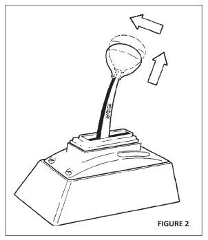
or DRIVE, lift the lever and move it to the NEUTRAL position. From REVERSE, simply pull the lever back into NEUTRAL.
