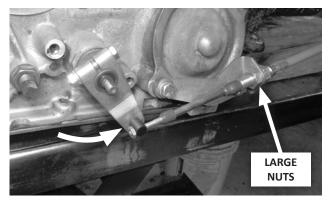
**34.** Manually move the selector lever to the LOW (full-rear) detent. Ratchet the shifter handle to the LOW position (furthest back). Adjust the large cable nuts until the swivel slides freely in and out of the hole in the selector lever. Gradually tighten the nuts against the bracket, while continuing to check the fit of the swivel in the selector lever.
