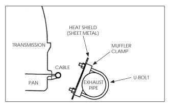
**CAUTION:** Heat will severely damage the shift cable, causing the housing to melt or become brittle. If the cable must be routed near exhaust system components, fabricate a heat shield. **Do not wrap the cable, as this retains heat.**
