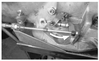
19. With the swivel still in the selector lever, move the shifter to the PARK (full-forward) position. Verify that the swivel still slips freely in and out of the selector lever. If not, adjust the large cable nuts (and the swivel, if necessary) until it does.
