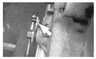
**55.** Secure the swivel to the selector lever with the cotter pin. Operate the shifter through all the gear positions, verifying that it operates correctly.
