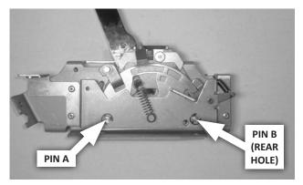
6. Configure the park and speed limiter pins for your application as shown in the photo and table. (Each pin is secured with two 1/4" e-clips.)
