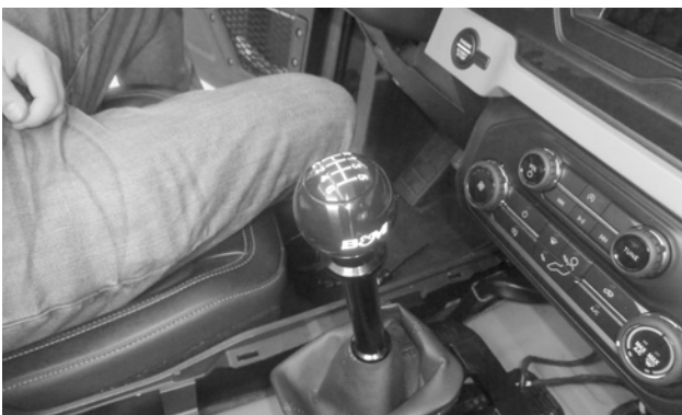
54. Snap the cap onto the shift knob.
