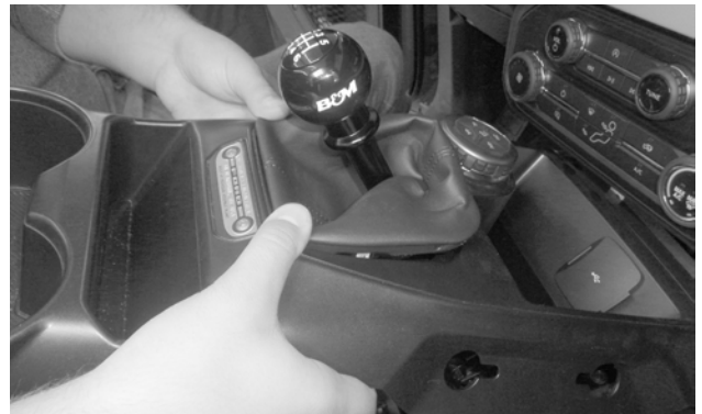
57. Snap the boot frame back into place in the console panel.
