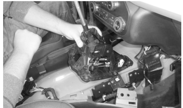
21. Remove the shifter assembly from the vehicle.
