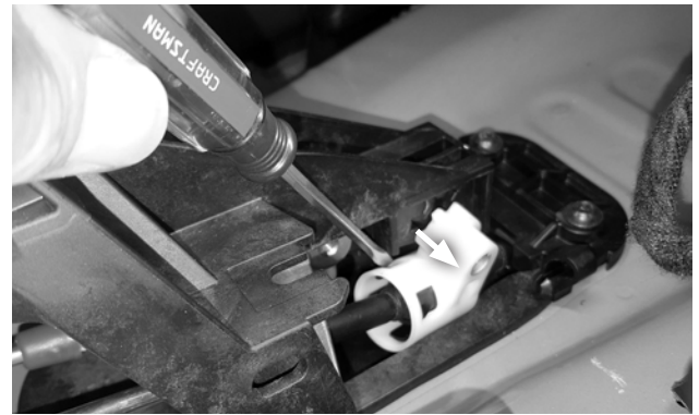
20. Disengage the 2 white cable bushings from the front of the shifter housing (1 on each side).
