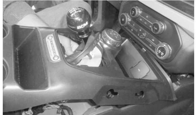
56. Carefully move the console panel into place above the center console. Feed the boot frame up through the panel opening.
