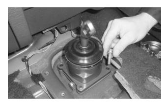
**14. Install the B&M shifter** using the stock screws. Tighten the screws to 17 ft-lbs torque.
