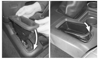
**19. Reinstall the transfer case lever boot** or the storage bin in the console rear half.
