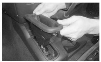
**3.** For vehicles with a manual transfer case lever, move the lever to NEUTRAL, then separate the boot from the console and lift it clear, to access the console screw underneath.
