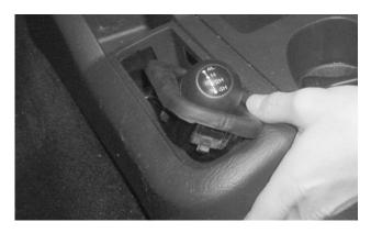
**NOTE:** For vehicles with a manual transfer case lever, tilt the boot frame slightly to fish it up through the opening.
