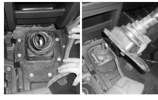
8. Remove the dust boot screws and the dust boot.
