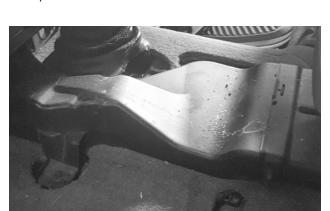
16. Reinstall the air conditioner / heater duct (if so equipped).
