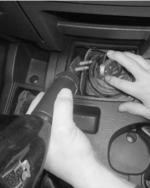
**2.** At the bottom of the shift lever, pull the dust boot down to expose the 2 nuts. Remove the nuts and the lever.
