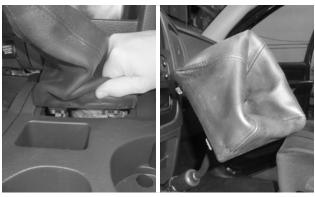
Shift the transmission to NEUTRAL. Separate the shift lever boot from the console, and slide the boot to the top of the lever.
