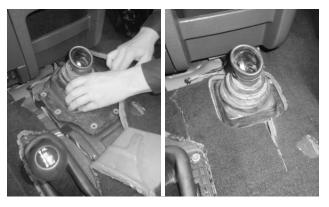
**15. Reinstall the dust boot** and screws, and return the carpeting to its place.
