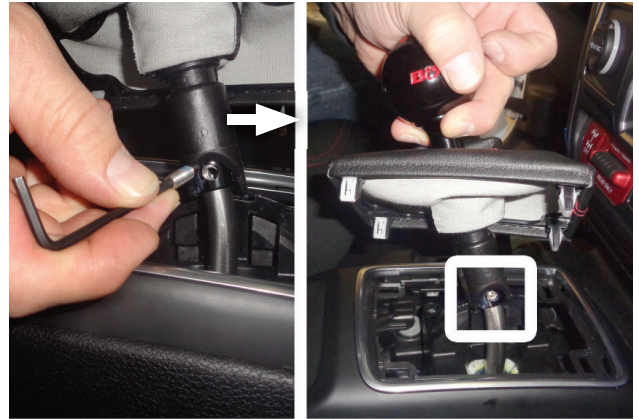
45. Apply blue permatex thread locker (or similar) to set screw (5) . Pull up on reverse lockout to expose and align parts at alignment hole in shifter stem, then install set screw as shown.
