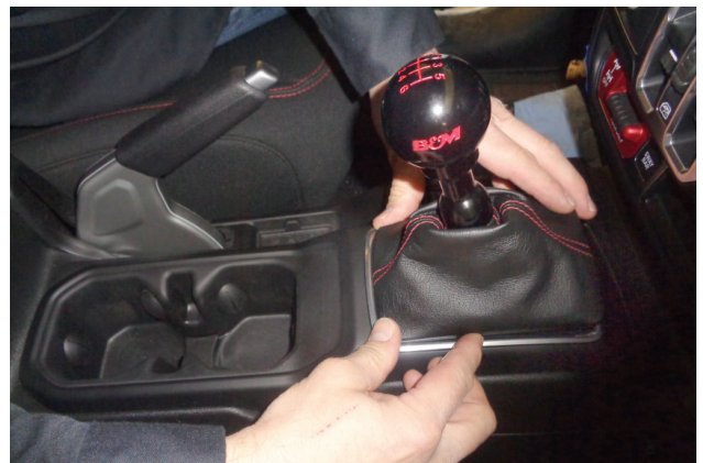
46. Set boot down into console in place.
