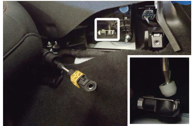
16. Disassemble lower cable from pivot cup, accessed on front passenger side of console.
