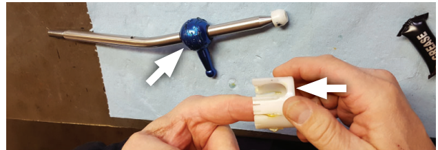
21. Apply grease from kit to pivot cup (removed step 20) and bottom pivot arm of shifter assembly (1) . Then install pivot cup onto shifter assembly.
