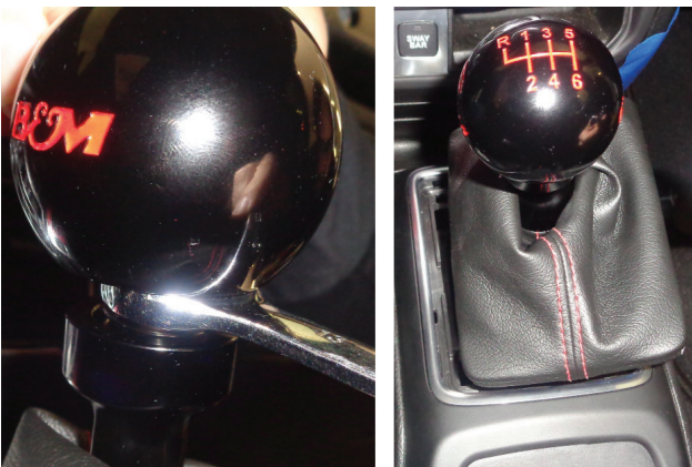
44. Turn knob back until it is aligned to your preference, then adjust jam nut to set knob in place.
