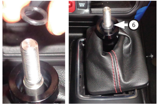
40. Install O-ring (6) onto shift stem so it rests in groove as shown.
