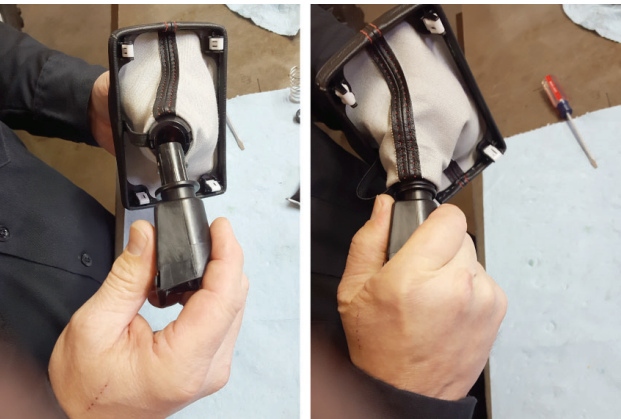
26. Insert reverse lockout factory bottom (removed step 24) into boot aligned with slot and press it into reverse lockout top until components click together.
