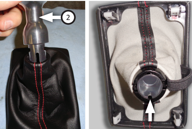
25. Align slot on reverse lockout (2) toward rear side of boot. Install reverse lockout into boot.
