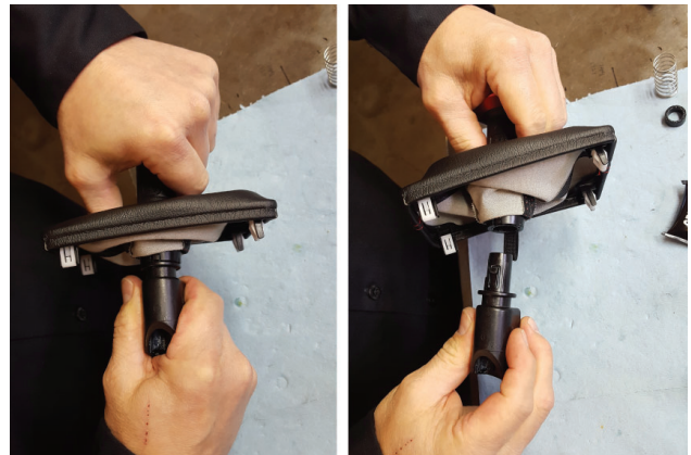
23. Pull factory reverse lockout bottom from stock shifter handle assembly (removed step 10) and retain it for later use.
