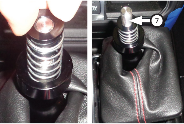
42. Thread jam nut (7) onto shifter stem then finger-tighten it fully.
