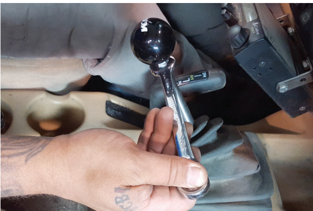
25. Adjust knob until it is in optimal position, then tighten it in combination with lock nut to secure it in place.
