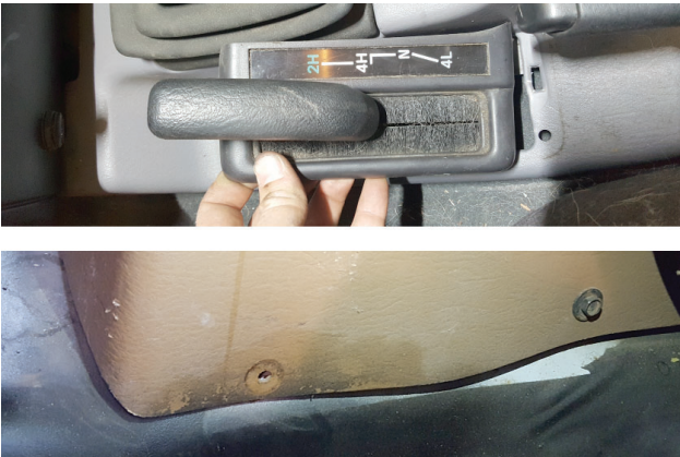
7. Remove 4wd selector cover or remove and retain fasteners securing passenger side of center console.
