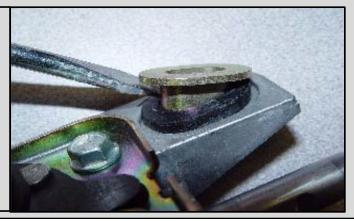
D. Install the provided spacers underneath the base as shown.
