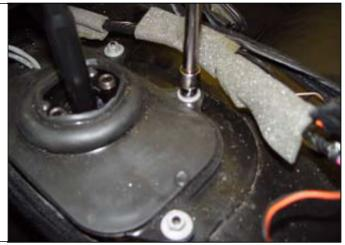
11. With the E-brake in the ON position, place the shifter in neutral and remove the 4 bolts securing the shifter to the transmission shifter base.
