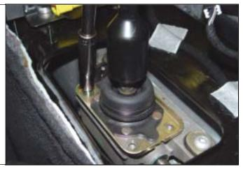
12. Gently remove the pivot cup from the bottom of the stick. For extra protection, use a towel between the channel locks.
