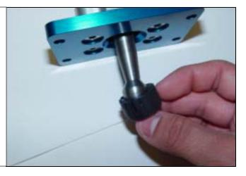
14. Remove the old rubber gasket completely and install the provided gasket.
