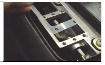
15. Install the B&M shifter. Secure the shifter to the transmission shifter base with the (4) provided 1/4" washers and 1/4"-20 screws. (Add a drop of medium-strength thread-locker (Permatex Blue or similar) to threads for added security.) Test shifter through all gears.
