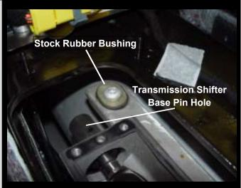
A. See top-right picture for indication of working area. Remove "L" pin from the stock shifter. With the shifter still in neutral and E-brake in the ON position, insert the "L" pin into the pin hole of the shifter base. The "L" pin is used to keep everything aligned. If done correctly, shifter should not be able to shift out of neutral position.
