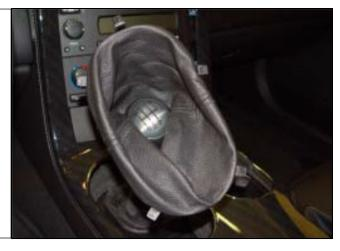
7. Hold top of knob and turn chrome collar counterclockwise to loosen collar and access bolt securing knob.
