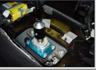
Reinstall the second rubber layer, securing the rubber using (4) nuts. Reinstall the first rubber layer.
