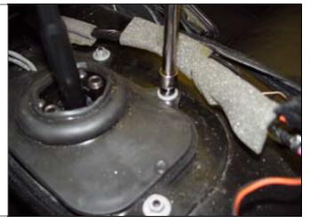
17. Reinstall all connector wires to the center console. Install the knob into the leather boot before installing back into the shifter (clip the knob back into the chrome collar). Reinstall the center console trim plate. Install the knob into the shifter.
