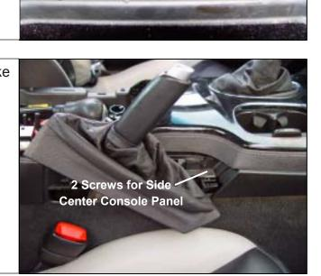
4. Remove the (2) bolts holding down front center console, located right next to emergency brake.
