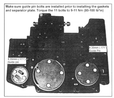
Figure 3. '96-'99 (TYPE B) Valve Body & Cover Plates
