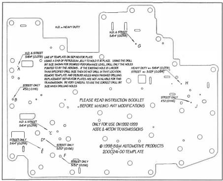
Figure 8. Separator Plate Drilling Template
