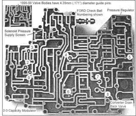
Figure 9. 1996-1999 Check Ball Placement (TYPE B Valve Body)
