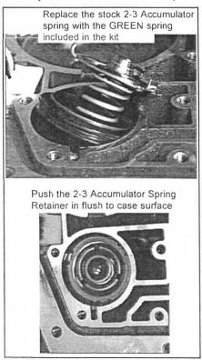
Figure 7. 2-3 Accumulator Assembly
