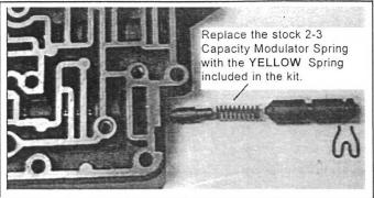
Figure 4. Pressure Regulator Spring
