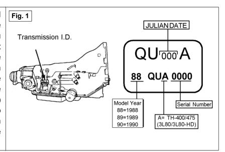
If the I.D. tag is unreadable or missing you will have to remove the oil pan and valve body from the transmission to determine if your transmission has an early or late style case (See Fig. 2). The manufacturing date check applies only to 1988 transmissions, this kit will work correctly in all subsequent application vears specified in the heading of these instructions.
