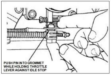
E. While continuing to hold the throttle lever against the idle stop, firmly push the pin on the cable adjuster all the way into the nylon grommet on the throttle lever.
