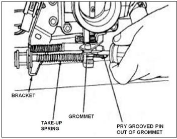
H. Remove gauge tool and pry grooved pin out of grommet on throttle lever.
