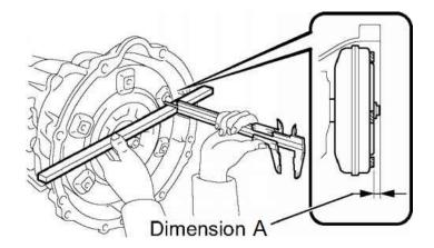
A. Measure Dimension A: While holding the torque converter in place against the transmission, use a straightedge to measure the distance between the bell housing mating surface and the torque converter mounting pads. (Typical AOD torque converter depth = 1", ±0.050".)
