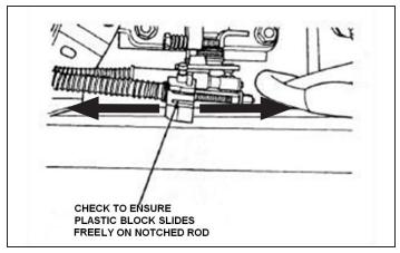
D. Verify that the adjuster block slides freely along the notched rod. If it does not slide freely, the white tab is not pushed out all the way.
