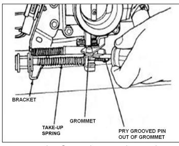
B. Use a large flat screwdriver to pry the grooved pin on the adjuster block out of the grommet on the throttle body lever.
