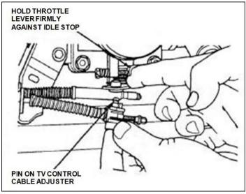
D. At the throttle body end, hold the throttle lever firmly against its idle stop.
