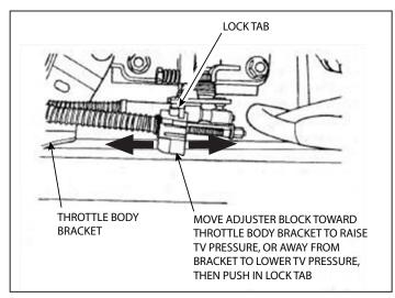
K. Using mark or measurement on the adjuster block as a reference, move block towards throttle body bracket to raise TV pressure, or move it away from bracket to lower TV pressure. Push in white locking tab to lock adjusting block in position.
