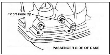
A. Attach TV pressure gage (0-60 PSI; Ford tool T86L-70002-A, or fabricate an equivalent) to TV pressure tap on passenger-side of transmission case.
