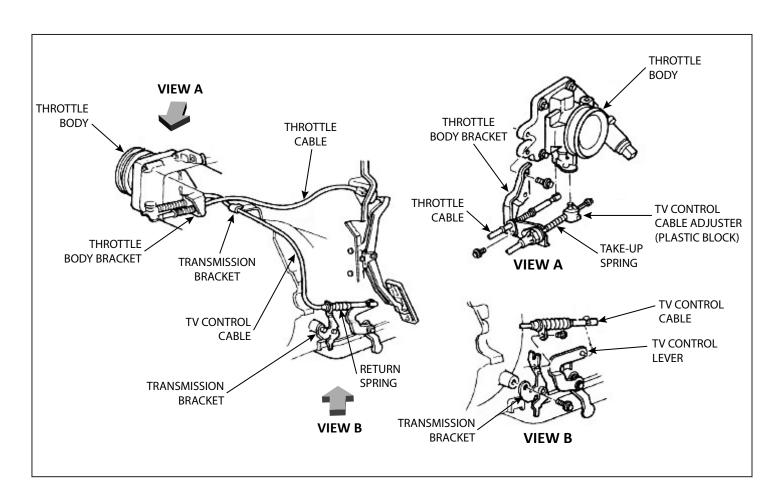
white locking tab is automatically pushed in, locking the cable to its correct length. After this, the take-up spring plays no part in the operation of the system.
