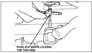
C. Use a small flat screwdriver to push the white locking tab all the way out.
