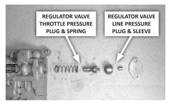
**48. Install the regulator valve group,** followed by its end plate (2 screws). Tighten the screws to 35 in-lbs.
