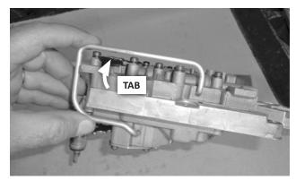
57. 4-SPEEDS: Install the boost tube, then bend the retainer tab(s) back into place against it. Go to Step 59.
