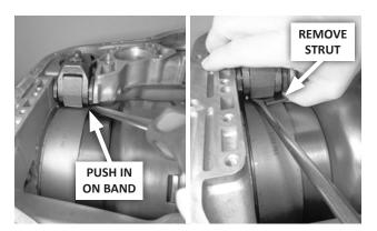
**71.** Use a long thin screwdriver to push in on the rear band. The band apply strut will pop out. Use a second screwdriver to remove the strut, then swing the apply lever clear of the servo.
