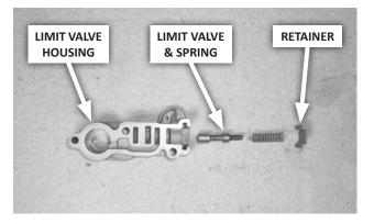
24. Disassemble the 3-2 downshift & limit valve assembly by removing the throttle plug (Step 23 photo), retainer, and limit valve group from the housing.
