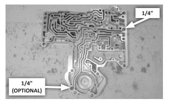
**20.** Carefully lift the stiffener, separator plate, and filter screen off of the transfer plate.
