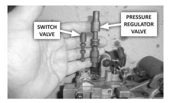
**14.** Remove the pressure regulator and switch valves. Note the orientation of the switch valve (large spool out).
