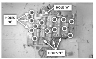
**56. 4-SPEEDS: Carefully lay the separator plate and lower valve body** on top of the transfer plate. Hand start, then tighten, 13 transfer plate screws. Tighten the screws to 35 in-lbs.
