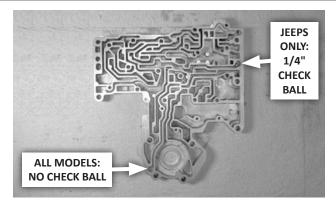
38. JEEPS ONLY: Install one 1/4" check ball in the transfer plate as shown.
