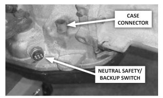
**83.** Install neutral safety/backup switch and tighten to 25 ft-lbs. Connect harness plug(s) to neutral safety/backup switch and case connector (if applicable).
