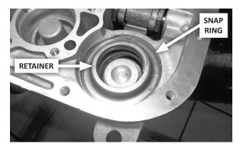
**72.** Compress the spring retainer, then remove the snap ring and retainer, followed by the spring and piston assembly underneath.
