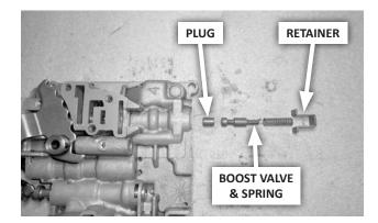
**46. 4-SPEEDS: Install the boost valve group,** followed by the cover plate (3 screws). Tighten the screws to 35 in-lbs.
