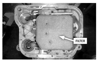
1. Drain and remove the transmission oil pan, then remove and discard the filter (3 screws). If your oil pan does not have a drain plug, consider installing B&M Drain Plug Kit 80250.
