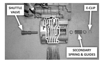
**47.** ALL: Install the shuttle valve group and e-clip. Verify ease of valve travel, then install its cover plate (6 screws). Tighten the screws to 35 in-lbs.
