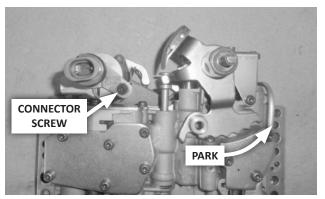
9. Move the selector lever to PARK (full counter-clockwise), to protect the manual valve and to avoid losing the detent ball during disassembly. Remove case connector screw (if applicable). Note the screw's unthreaded shank, which permits connector "float."
