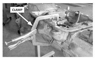
**CAUTION:** Avoid injury or lost parts! The rear servo piston spring is very strong. The spring retainer must be compressed until the snap ring is fully removed from its groove. A jack or clamp is recommended for both disassembly and reassembly.
