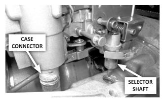
**81.** Carefully work the valve body the rest of the way into the transmission, paying special attention to selector shaft and case connector (if applicable) and their bores.
