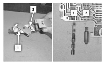
**32. 4-SPEEDS: Remove the end plate** (3 screws), then remove the #1 (3-4 timing) and #2 (3-4 quick fill) valve groups.
