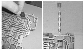
**30. 4-SPEEDS: Remove retainer and valve group #5, the converter clutch timing valve.** (Your valve group may include a spring; photo shows no spring because the transmission is non-lockup.)
