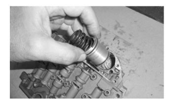
**28. 4-SPEEDS: On the lower valve body,** remove the 3-4 accumulator cover plate (5 screws), spring, and piston.
