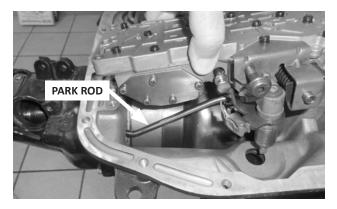
6. Carefully remove the valve body from the transmission, tapping gently on the case connector (if applicable). When the selector shaft and case connector are clear of the case, move the valve body forward to pull the park rod past the park pawl in the tail housing.
