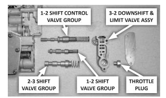
23. Remove the 3-2 downshift & limit valve assembly and end plate (3 screws).
