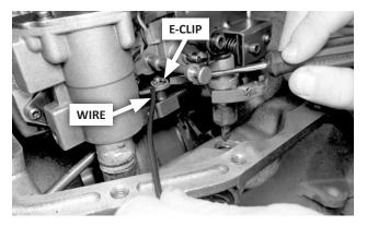
80. Secure the park rod pin to the selector lever with the e-clip.
