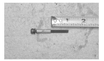
**43. 4-SPEEDS:** Wrap masking tape 1" from the tip of a valve body screw as a depth guide.
