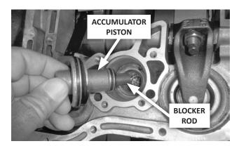
**69. ALL: Remove the accumulator piston from the case,** and insert the **blocker rod [12]** in the middle of the piston. Then install the piston and blocker rod in the case.
