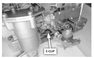
**8.** Move the valve body to a clean work surface. Remove the e-clip and park rod.
