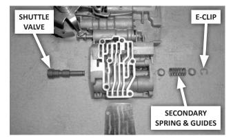
26. Remove the shuttle valve cover plate (6 screws), followed by the e-clip, shuttle valve, secondary spring, and spring guides.
