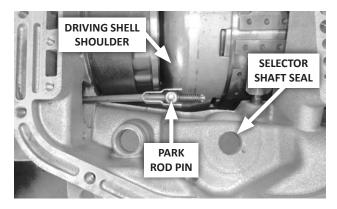
**78. Insert the park rod through the case opening** and past the park pawl. The pin at the front of the rod should be about even with the shoulder of the sun gear driving shell.
