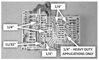
53. Install the steel check balls as shown.
