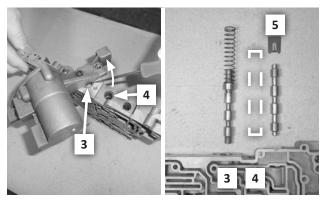
**31. 4-SPEEDS: At the 3-4 accumulator housing, remove the 2 end screws.** Then loosen the center screw, and pivot the housing slowly to release first the #4 valve group (converter clutch valve), then the #3 valve group (3-4 shift valve). (Photo shows no #4 valve group because the transmission is non-lockup.)
