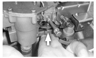
**79.** Lubricate the selector shaft, case connector o-rings (if applicable), and their case bores with assembly grease or transmission fluid. Move the selector lever to LOW (fully clockwise) so it will reach the park rod. Move the valve body close to the transmission, then insert the park rod pin into the selector lever hole. Do not insert the selector shaft or case connector into their bores yet.
