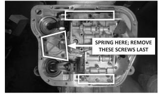
5. Detach the valve body from the transmission (10 hex screws).
