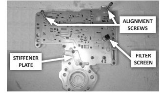
**39.** Insert the filter screen in the separator plate, then lay the separator plate on the transfer plate. Temporarily thread 2 valve body screws into the locations shown to align the separator and transfer plates, then attach the stiffener and separator plates to the transfer plate with the screws removed at **Step 19**. Be sure to orient the stiffener plate the same way as when it was removed. Tighten the screws to 35 in-lbs, then remove the 2 alignment screws.
