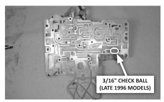
**55. 4-SPEEDS:** If a 3/16" check ball was removed at Step 17, install it in the oval pocket on the transfer plate as shown.
