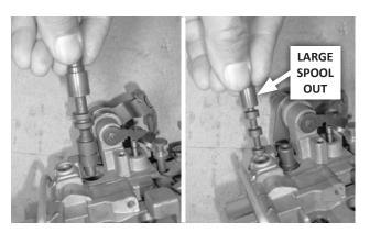
**61. Install the pressure regulator valve and B&M spring (6),** then the switch valve (large spool out) and spring.
