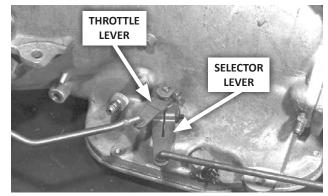
Loosen the selector lever pinch bolt, move the vehicle's shifter to LOW, and remove the lever from its shaft. Carefully move the lever and shift rod aside, allowing them to hang free.
