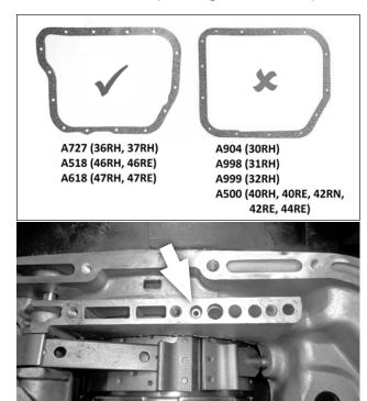
**Install the steel orifice plug [14]** in the hole indicated. The edge of the plug must sit just below the case surface.
