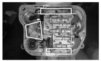
**82.** Secure the valve body to the transmission (10 screws). First run the screws in finger-tight, and verify the valve body sits flat against the case. Then tighten the screws in an alternating pattern to 100 in-lbs.
