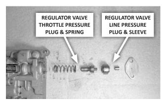
**25. Remove the regulator valve end plate** (2 screws), followed by the regulator valve group.
