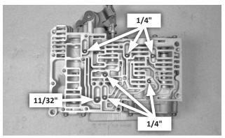
**18.** Note the location and size of the 7 check balls in the valve body casting, then remove them.
