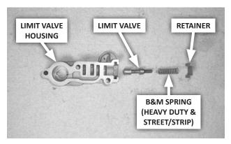
49. Assemble the 3-2 downshift & limit valve assembly.
