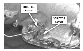
**84. Connect the shift linkage and throttle linkage** to the transmission (reverse of **Steps 3 & 4**).
