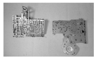
**17. ALL: Carefully lift the transfer plate assembly** off of the valve body casting, and set it aside with the separator plate facing up.
