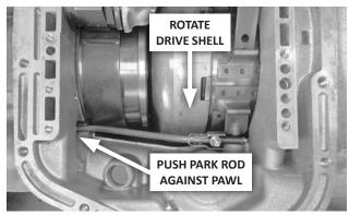
**NOTE:** If the transmission hasn't been rotated since removal of the valve body, the park rod should easily slip past the park pawl. If it doesn't, rotate the drive shell counter-clockwise (viewed from the front) while pushing the park rod against the pawl, until the rod is fully inserted.
