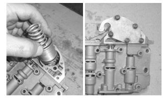
**45. 4-SPEEDS: Install the 3-4 accumulator piston and B&M spring [9]** in the lower valve body housing. Then install the accumulator cover (5 screws). Tighten the screws to 35 in-lbs.
