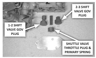
22. Remove the governor plug end plate (5 screws).
