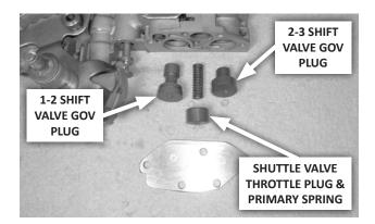
**52. Install the 2-3 shift valve governor plug,** shuttle valve throttle plug & primary spring, and 1-2 shift valve governor plug, followed by the governor plug end plate (5 screws). Tighten the screws to 35 in-lbs.
