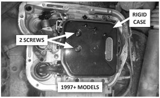
**NOTE:** If your filter has a rigid case and is attached with 2 screws, your transmission is a 1997 or newer. **STOP, this kit is not compatible!**
