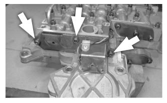
11. 4-SPEEDS: Remove solenoid & harness assembly (3 screws).
