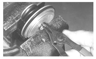
**73.** Use a vise to compress the spring slightly. Remove and discard the snap ring, then disassemble the piston.
