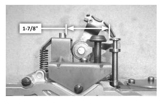
**63. Verify bracket alignment:** Distance from the edge of the manual selector valve to the pressure adjusting screw must be 1-7/8". If not, loosen the 3 screws, adjust the bracket, retighten the screws, and re-measure.
