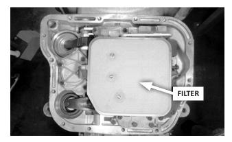
**85.** Install the new B&M filter [5] (3 screws). Tighten the screws to 25 in-lbs.
