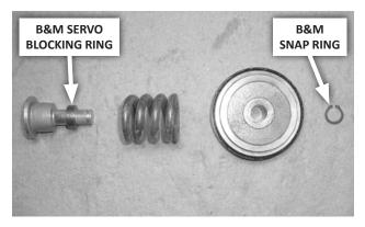
74. Install the servo blocking ring [16] over the servo shaft, then reassemble the piston, using the B&M external snap ring [15].
