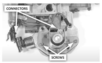
**10. RE MODELS: Remove the connectors** from the governor pressure solenoid and governor pressure sensor. Then remove governor pressure housing, retainer and gasket (2 screws).
