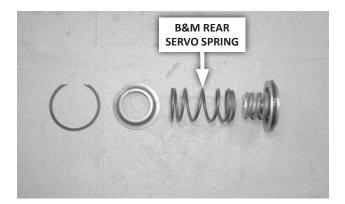
75. Install the rear servo piston in the case, taking care not to damage its rubber lip seal. Then install the B&M rear servo spring [11], compress the spring retainer (a jack or clamp is recommended), and install the snap ring.
