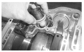
7. Remove the 1-2 accumulator spring and piston, and discard the spring.
