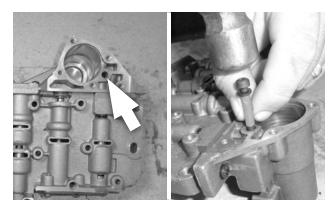
**44. 4-SPEEDS: Use the screw to gently tap the B&M aluminum orifice plug [13]** into the oil passage next to the 3-4 accumulator bore. Seat the orifice plug 1" below the machined surface.
