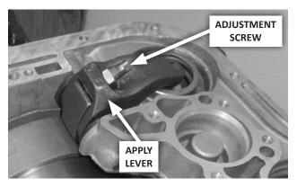
**70.** Loosen the rear (low/reverse) servo band adjuster locknut, then back the adjustment screw out until the tip is flush inside the apply lever (typically 3-4 turns).
