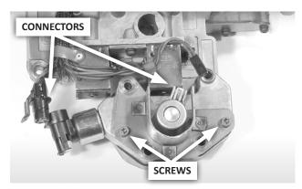
**67.** If applicable (RE models), install the governor pressure housing, retainer and gasket (2 screws; tighten to 35 in-lbs). Connect the harness to the governor pressure solenoid and sensor.
