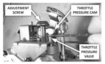
65. Adjust the throttle pressure screw so that the 1/8" drill bit[20] just fits between the throttle pressure cam and throttle pressure valve.
