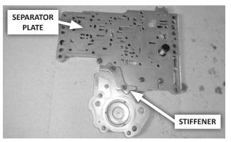
**19.** Note the orientation of the stiffener, then remove the 4-6 screws (varies by model) attaching the stiffener and separator plate to the transfer plate.
