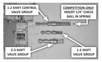
**50. Install the 2-3 shift valve group,** 1-2 shift valve group, and 1-2 shift control valve group in the valve body.
