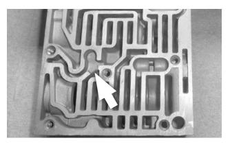
**35. Remove the section of casting wall as shown** by drilling through the hole in the guide.
