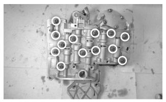
**15.** Remove the 13 valve body screws (and boost tube retainer, on 4-speeds).
