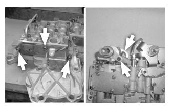
**66. Install the solenoid & harness assembly, if applicable** (3 screws; tighten to 35 in-lb). Route the wiring through the 3-4 accumulator cover plate, then attach the case connector with the shoulder screw (tighten to 35 in-lbs).
