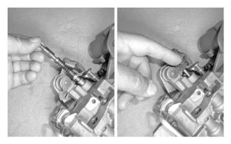
**60. Install the throttle valve group** in the valve body. Then pivot the throttle pressure lever back into place against the valve.
