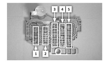
**29. 4-SPEEDS: Lay the lower valve body flat** with the accumulator housing at the top left corner. Note the 5 valve group locations as shown.
