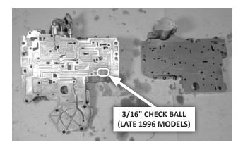
**16. 4-SPEEDS: Carefully lift the lower valve body** and separator plate off of the transfer plate, and set them aside.
