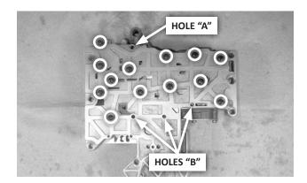
**58. 3-SPEEDS: Hand start, then tighten, 13 transfer plate screws.** Tighten the screws to 35 in-lbs.
