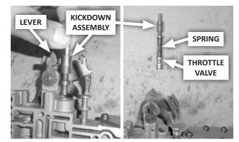
**21.** Pivot the throttle pressure lever upward, and remove the throttle valve group (kickdown assembly, spring, and throttle valve).
