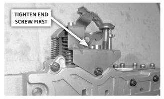
62. Move the spring retainer & adjusting screw bracket into place, capturing both the switch valve and pressure regulator springs. Push the bracket down against the springs, align the screw holes, and hand start all 3 screws. Tighten the end screw first, followed by the 2 side screws (35 in-lbs).
