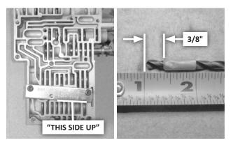
**34.** Install the B&M drill guide [item 17] on the valve body casting as shown, using 2 end plate screws. Wrap masking tape 3/8" from the tip of the 3/16" drill bit [18] as a depth guide.
