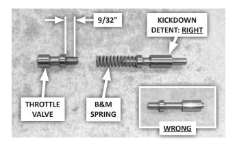
59. ALL: Grind the throttle valve stem to 9/32" long and deburr. Then reassemble the throttle valve group using the B&M throttle pressure spring [7]. Ensure that the kickdown detent is correctly installed on the kickdown valve as shown.
