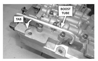
**12. 4-SPEEDS: Bend tab(s) down on boost tube retainer.** Then carefully pull the boost tube out of the valve body.
