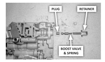
**27. 4-SPEEDS: Remove the boost valve cover plate** (3 screws), followed by the boost valve group.
