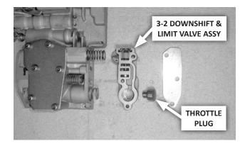
**51.** Install the throttle plug in the 3-2 downshift & limit valve assembly, then install the valve assembly and end plate on the valve body (3 screws). Tighten the screws to 35 in-lbs.
