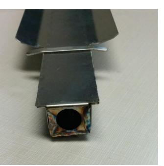
To ensure the burner is properly Seated, locate the orifice hole and the orifice (3). In the end of the burner there is an opening for the orifice to enter (2). Slide the burner opening onto the orifice (3) and secure to the burner bracket. NOTE: the burner will not align with the burner bracket if it is not properly seated onto the orifice
