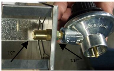
5. Using threadlocker on the threads, screw the new orifice back onto the fitting and tighten. Re-assemble BBQ
