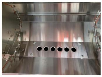
2. Remove the nut holding the burner in the unit, pull the burner to the left and slightly up and remove.
