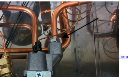
5. Remove the broiler connection at the back of the stove. Use a pair of vice grips to brace the fitting when undoing the compression fitting with a 9/16" wrench.
