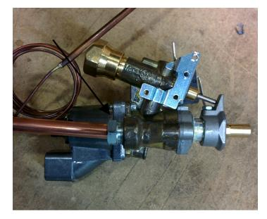
8. Follow directions 1-6 in reverse order to re-install the new valve. Make sure to use a thread sealant on all gas connections.
