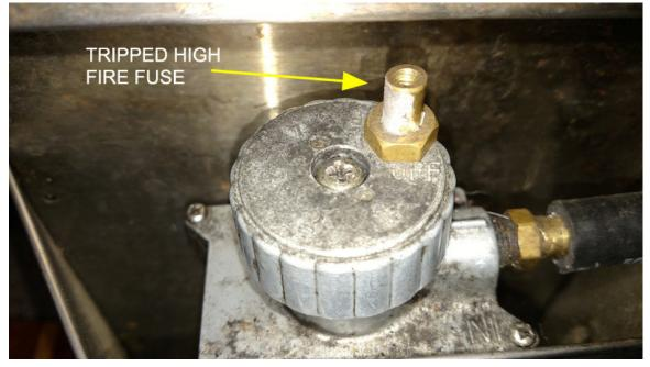
If this happens then you have 2 options. Option 1 is to replace the fuse with a new one. To do this you would remove the old fuse by unscrewing the brass nut that contains the assembly. Then you would screw in the new fuse tightly and then calibrate your fuel flow.
