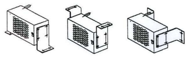
Using the "Side Mount Bracket Kit" for the Radex, you can mount the unit to a wall, floor or ceiling in a number of different ways.
