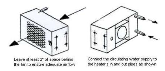
After the fan wiring and water installation are complete, secure the Radex in the mounted position with the desired mounting kit.
