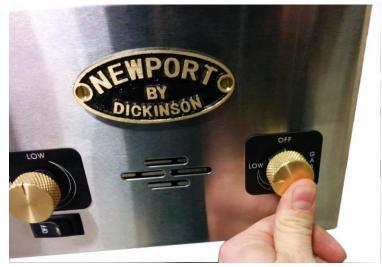
5) Close the door and hold the knob in for an additional 15 seconds to allow the thermocouple time to engage the valve
