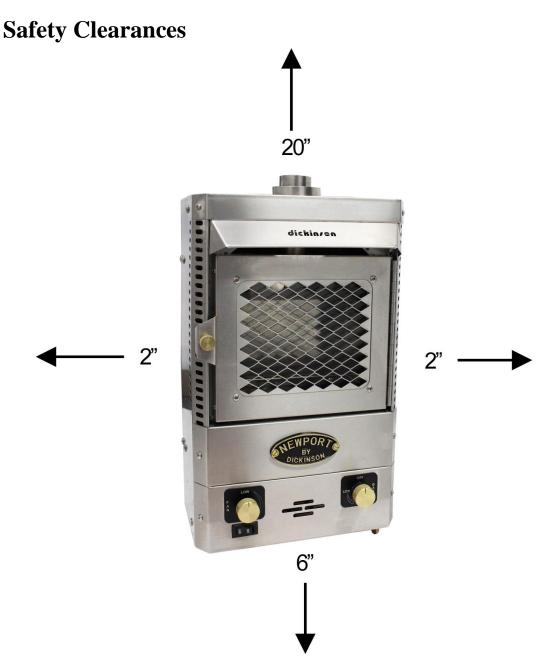
Combustible material such as the deck/ceiling or walls that are closer to the heater then the specified safety clearances must be insulated with insulation or cement board with a metal liner, a .5" standoff is best for air movement behind. Another alternative is using insulation or cement board and ceramic tile.
