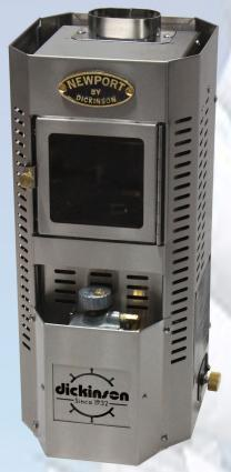
Fuel Consumption / 24hrs 1.29Gal Low High 3.20Gal **Heat Output** Low 6500 BTU High 16250BTU Width 8.5" Depth 10.5" Height 19.75" Weight 22lbs (10Kg)
