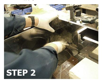
${f 2a.}$  Spread the cement around the stove evenly, about a half an inch thick, and use a trowel to smooth out the surface.
