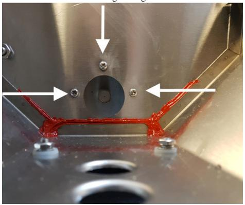
5. Using a small needle or drill bit, clean out the small hole in the end of the orifice.
