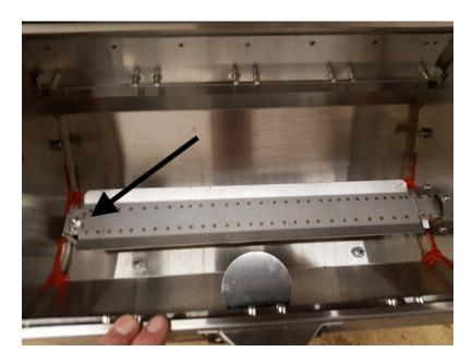
3. Pull the burner to the left and up to remove.
