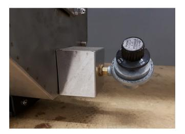
5. Place the left end of the burner over the exposed screw, tighen the nut back and replace the grills.
