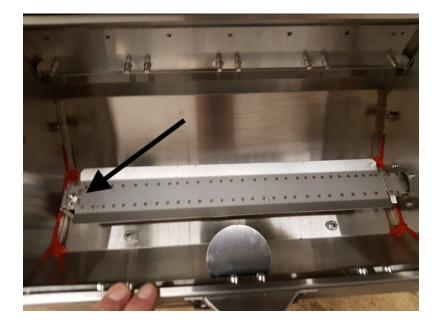
3. Pull the burner to the left and up to remove.
