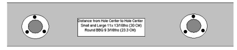
2. Once the holes are drilled insert the sockets and secure them to the rail with the  $6 \# 12 \times 34$  wood screws
