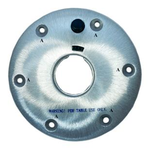
1. Identify where you are going to install the mount on the deck and attach the pedestal mount base to the deck by securing all the mounting holes (A) with deck screws. The base has an overall diameter of 7" and the ring of mounting holes has a diameter of 5.75"
