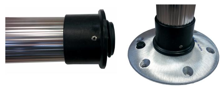
2. Once the pedestal mount base is secure, twist the base of the pedestal mount column into the base. Turn the column clockwise until it will not turn anymore.
