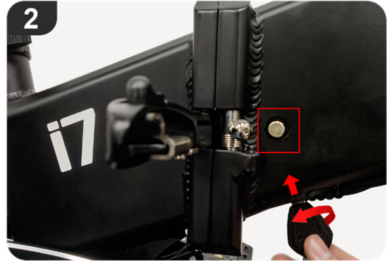
2. Push the key up once, then turn the key to retract the lock.
