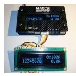
If the Hub X8 is installed in a place where the display is no more visible, then you can connect here a standard 2x16 LCD display (4-bit data bus), but please do not use any LCD displays with back LED light, as these lights can draw easily more than 200mA and the supplied power from the Power-Cube might be not enough.
