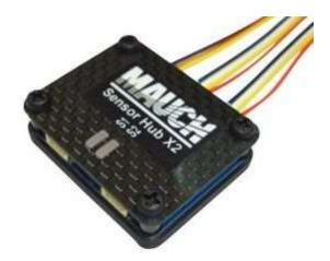
This sensor hub is to connect two PL-xxx current sensors in parallel. The current of both sensors will be summarized and passed to the FC. The voltage measurement of the LiPo packs will be collected from both sensors and passed through the Hub to the FC.
