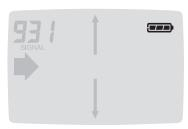
**3. Left/Right & Over-Target:** These indicators show your position relative to the center of the electromagnetic field.
