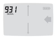
2. Battery Strength: When battery life declines to less than 1 hour (estimated) of operation the battery indicator outline will be illuminated with
