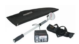
The Fisher M-101 metal detector was designed specifically for finding reinforcing bars and other metal objects embedded in concrete, conduits, PK nails, wiring, wall studs and other metallic objects. Users may expect accuracy to 1/4" of the centerline of the rebar.
