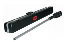
The Fisher FX-3 Ferro Probe senses fluctuations in the earth's magnetic field caused by buried survey markers, pipes, well casings, valves, iron relics, septic tanks and other ferromagnetic (iron or steel) objects. Because it's a differential-induction magnetometer, the FX-3 locates buried iron objects far beyond the reach of ordinary (search-coil-type) metal detectors.
