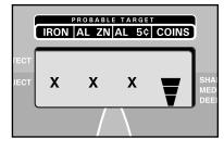
progressively eliminated, from left to right on the display. When all three "X"s are illuminated, the next press will erase all "X"s, returning the detector to all-metal detection status, where all types of metals will be detected.
