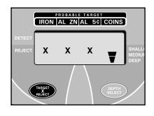
right, the common, less desirable, targets. When all three "X" are illuminated, the next press will erase all "X"s, returning the detector to all-metal detection status, where all types of metals will be detected.
