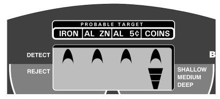
The four categories depicted across the top of the display indicate the probable identification of buried, detected metal objects. The searchcoil must be in motion over an object to be detected. Alternatively, you can pass an object over a motion less searchcoil to test your detector. One of the four target indicators will illuminate, indicating the probable identification of the object. The indicator will remain illuminated until another object is detected.
