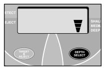
When three segments are illuminated, the detector is at maximum sensitivity. As you press the DEPTH SELECT touch pad, the detector toggles among the three different sensitivity levels. A more detailed explanation of depth selection is found on page 14.
