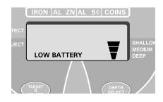
rates. When LOW BATTERY illuminates, it is possible that only one of the batteries requires replacement.
