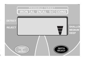
the detector among three different sensitivity settings. The detector is at maximum depth capability when three depth segments are illuminated on the right of the display.
