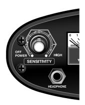
Sensitivity will be reduced slightly when using the Pioneer 101 in the Tone Discrimination mode. If you want optimal depth capability, operate in the All Metal mode by turning the Discriminate control completely counterclockwise; then turn the Sensitivity control clockwise to its highest clockwise position without chatter. If your Pioneer 101 chatters or beeps erratically, reduce the Sensitivity by turning the left knob counterclockwise.
