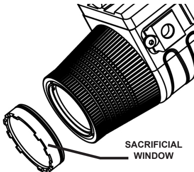
Figure 2-5 Sacrificial Window Installation
