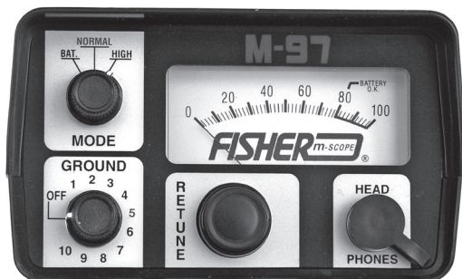
M-97 Control Panel
