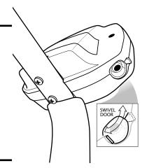
Using a detector with headphones facilitates detection of the weakest signals and also extends battery life.
