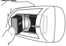
**If batteries fit too tightly**, causing battery door to bulge, move battery wires toward front of compartment, not between the batteries.
