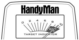
If the needle does not enter the green zone, replace the batteries.
