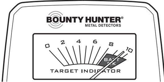
If the needle does not enter the green zone, replace the batteries.
