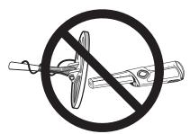
To minimize interference while probing the ground, lay the metal detector down with the searchcoil perpendicular to the ground.
