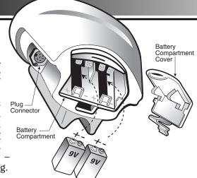
Insert (2) 9-Volt **ALKALINE**batteries, with the contacts pointed inward, and press down on the back of the batteries to snap them into place.
