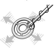
When pinpointing a target, try drawing an "X", as illustrated, over where the tone is induced.
