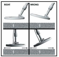
9. The diagram below shows the search coil detection pattern
