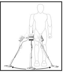
When the stem length is properly adjusted, the 1225-X is balanced for sweeping in a tight semicircle. Always overlap your sweeps by at least 50% or you'll miss a lot of the deeper targets. 1. For very strong signals, you may improve your motion mode pinpointing accuracy by adding one or more of the following steps:
