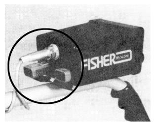
Figure 8. Battery Replacement
