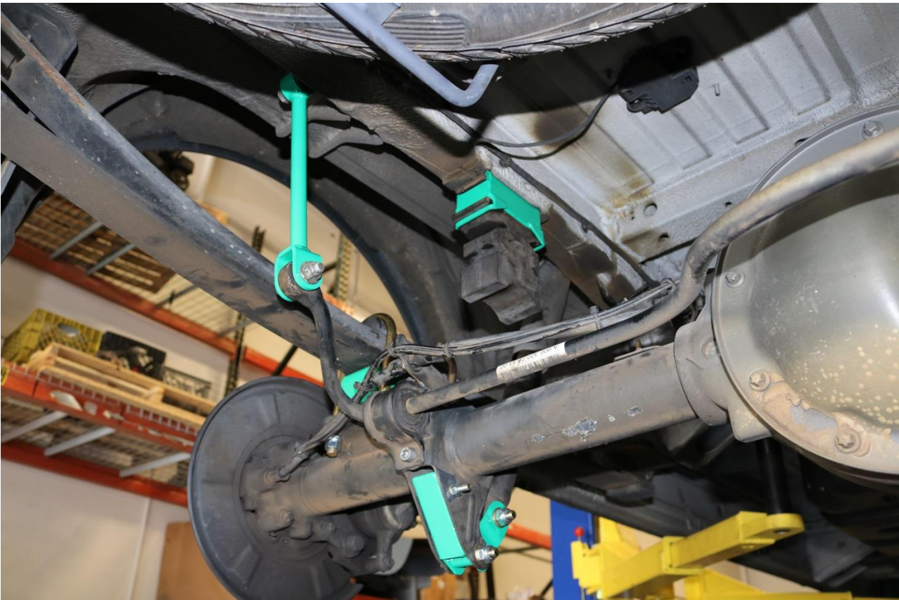
31) Cut the 3/8" ID rubber vacuum hose included with the 4008 Rear Brake Line Drop Bracket kit into two equal length pieces. Position a piece over each brake hose where it touches the leaf spring. Split the
