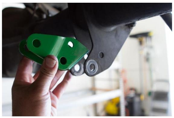
36) Install the M12-1.5 x 70MM long bolt and M10-1.5 x 65MM long bolt in their corresponding hole locations. Fit the 300301-03 Spacer bung in the shock mount prior to installing the M12 bolt. Be sure to use a washer under both the bolt head and nut on all bolts. Do not tighten hardware at this time.
