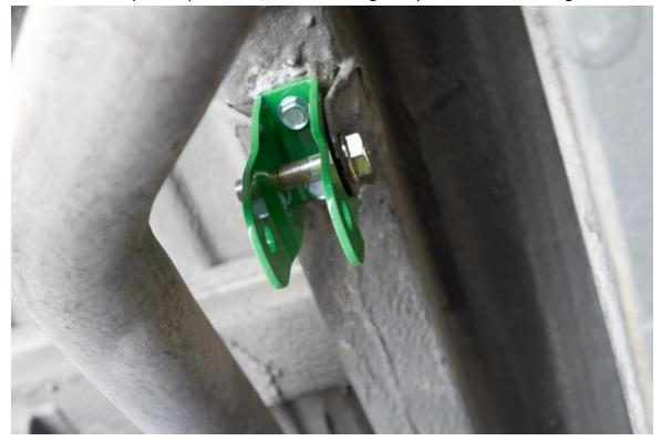
28) Use drill / driver to snug bolts into place. Do not fully tighten using drill / driver. Torque bolts to 13 ft-lbs (17 N.m).
