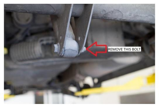
5) Fully remove the sway bar from the axle by using a 13mm socket and wrench to disconnect the 4 sway bar attachment bolts at the axle. Carefully remove the sway bar from the vehicle to not damage the e-brake and ABS sensor cable.
