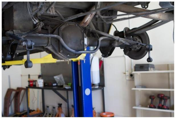
4) Support the axle and disconnect the lower shock bolt. Use an 18mm socket and wrench for removal. Once the shock is removed, allow the axle to hang freely again. Note that the springs will limit the downward travel with the shocks removed.
