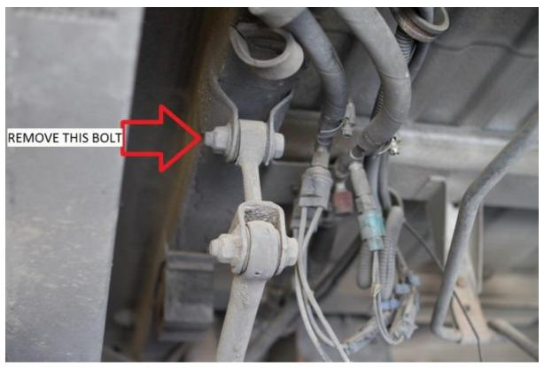
b. With the sway bar links disconnected from the chassis, allow the sway bar to rotate down as shown in the image below.
