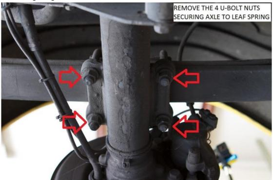
9) Lower the rear axle on the driver's side until there is approximately 2-1/2" (65mm) between the axle spring perch and the bottom of the leaf spring. Install the lift block so the pin on the lift block drops into place on the axle spring perch as shown below.
