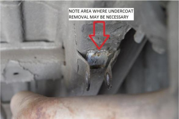
25) Install M12-1.5 x 55mm long bolt provided as shown above to locate bracket in place. Mark the two additional mounting hole locations which either a sharpie or transfer punch.
