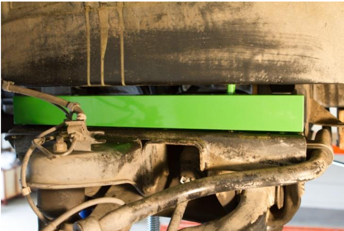
26) Install the drop spacer and jack up the sub frame until the drop spacer contacts the chassis as shown.
